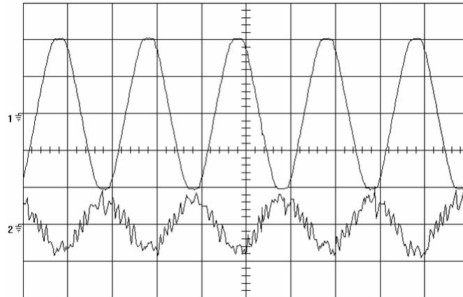
Figure 12. Regenerative operation of the line-side converter observed at generator load test (upper trace: phase voltage-110V/div, phase current-4A/div, time/div: 10ms)
