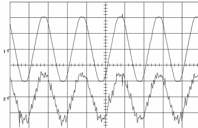
Figure 10. Rectifier operation of the line-side converter observed at motor load test (upper trace: phase voltage-110V/div, lower trace: phase current-4A/div, time/div: 10ms)
