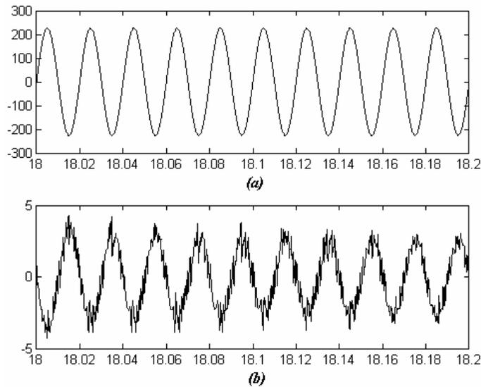
Figure 13. Simulation results for regenerative operation of the line-side converter (a) DCIM phase voltage (V) (b) phase current (A)
