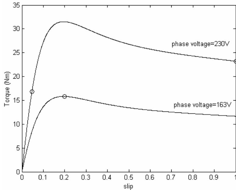
Figure 5. Steady-state torque-slip curves at rated and reduced armature terminal voltage. Continuous lines show the curve obtained from estimated parameters while the dots show measured values.
