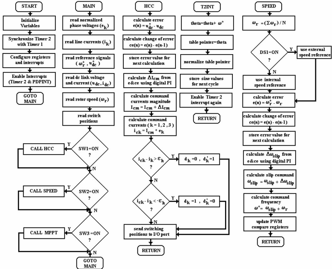
Figure 9. Flow-chart of the developed control software
