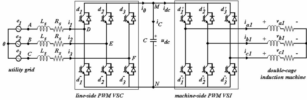
Figure 6. Electrical circuit of 3-phase PWM ac-dc-ac converter
