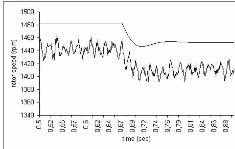
Figure 3. Speed response of the machine during transition from light load to normal load (upper trace-simulation, lower trace-experimental)
