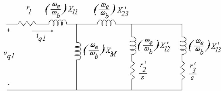
Figure 2. Equivalent circuit of double-cage induction machine
