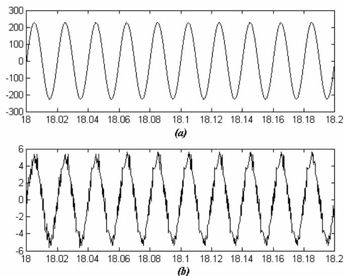
Figure 11. Simulation results for rectifier operation of the line-side converter (a) phase voltage (V) (b) phase current (A)
