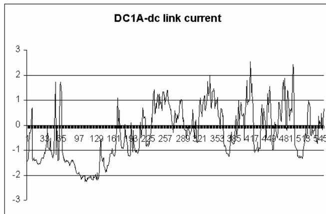
Figure 16. Recorded dc link current at a rotor speed of 940 rpm
