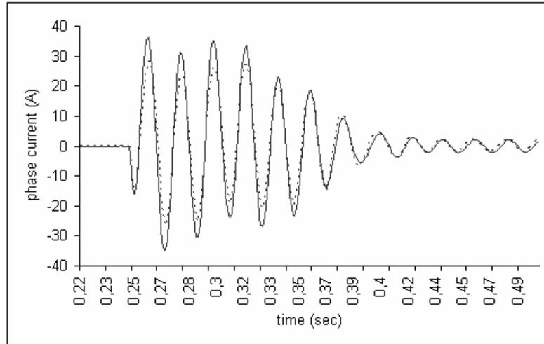
Figure 4. Phase current of the machine during free acceleration test (dotted lines-simulation, continuous lines-experiment)
