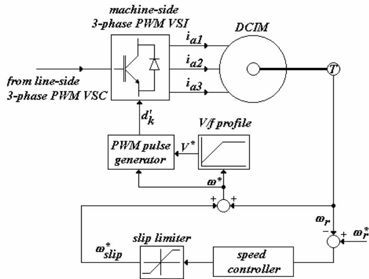
Figure 8. Closed-loop speed control scheme of the DCIM
