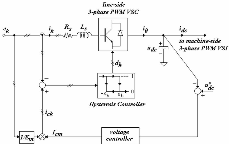
Figure 7. Closed-loop control scheme of 3-phase PWM ac-to-dc converter
