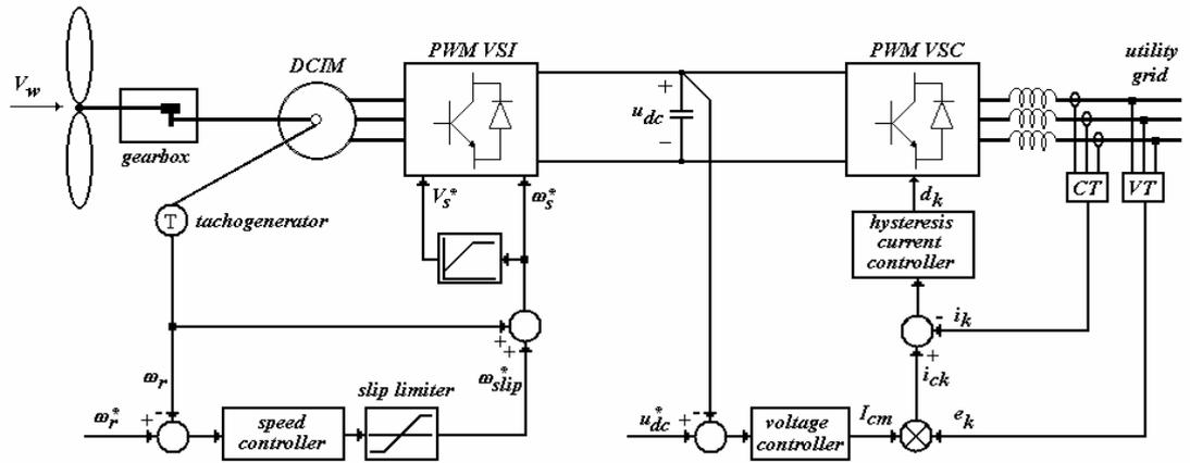
Figure 1. Variable speed wind generation system
