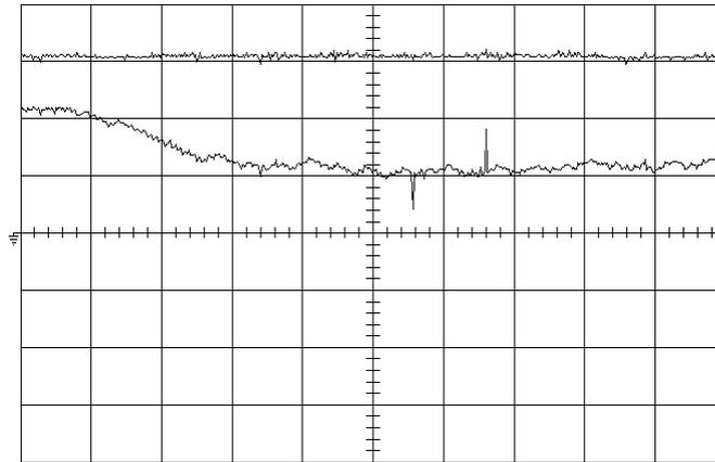
Figure 14. Experimental results during MPPT operation (upper trace: dc link voltage-160V/div, lower trace: rotor speed-375rpm/div, time/div-10s)
